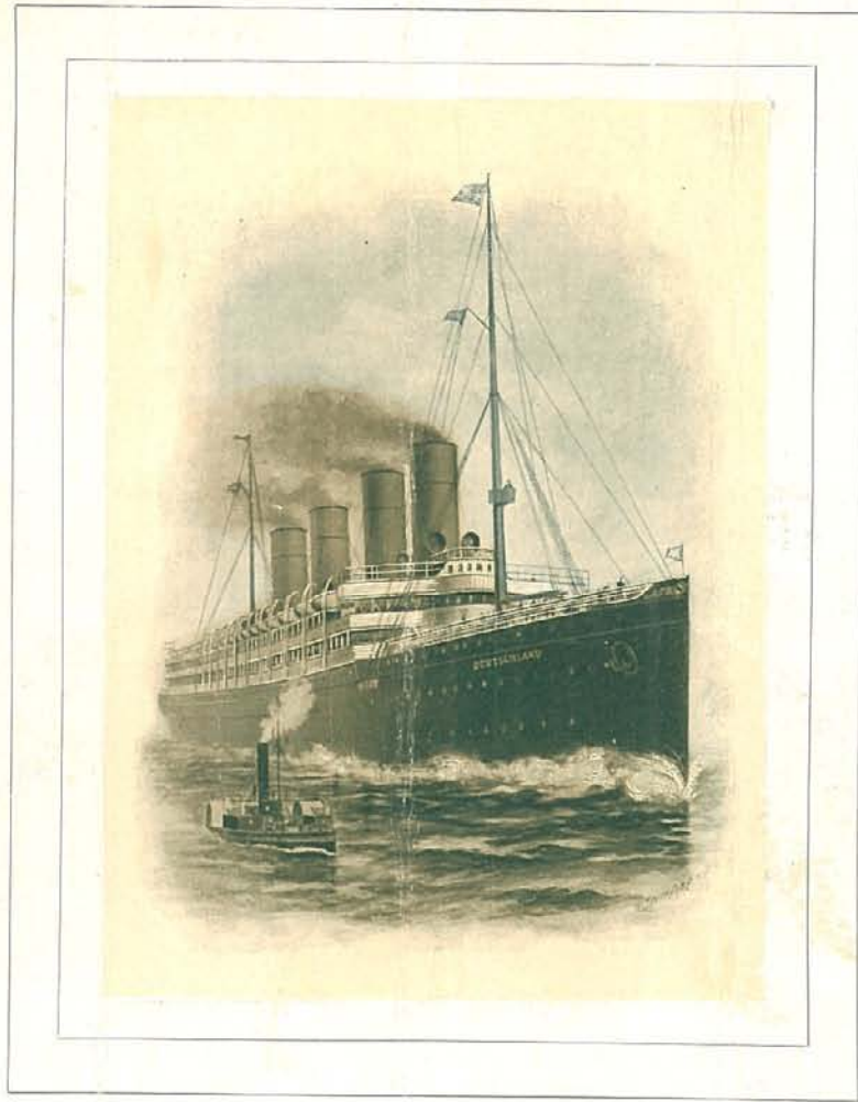
TWIN-SCREW EXPRESS S. S. DEUTSCHLAND, 16,000 TONS, 35,000 HORSE POWER, 23 KNOTS PER HOUR, 686 1-2 FEET LONG, 87 1-2 FEET WIDE.
